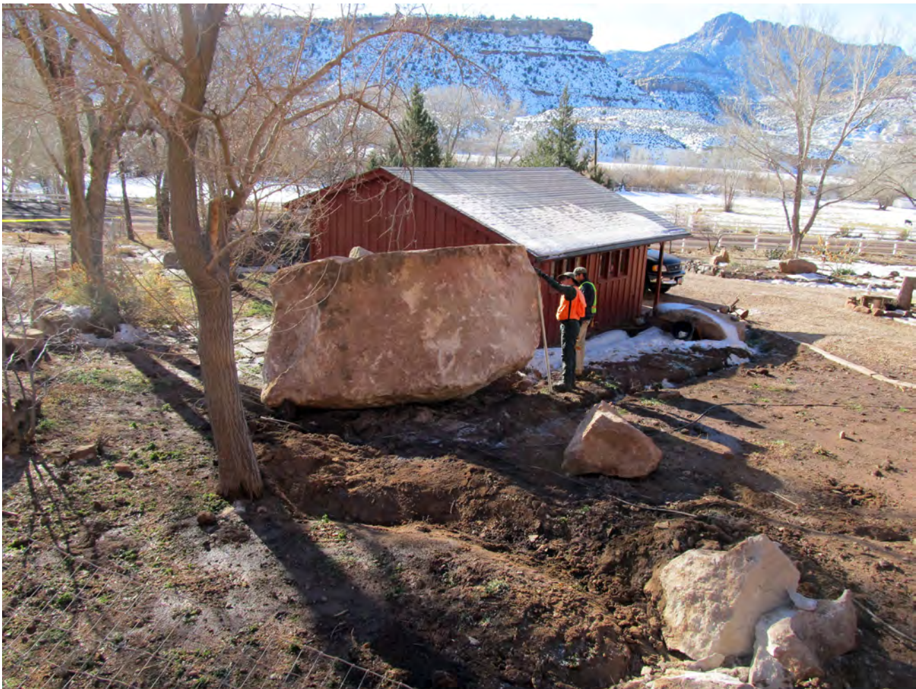
Figure 18. Largest boulder to reach the property immediately west of the December 12, 2013, rock-fall site. The boulder has an estimated volume of 21 yd 3 and mass of 41 tons; average boulder dimensions are 7.5 x 11 x 7 feet. Photograph taken on December 17, 2013, view is to the southwest.
